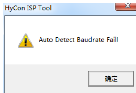
Figure 5. Auto-baudrate detect failure
